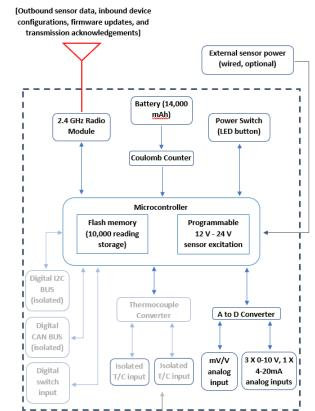
[0-10 V sensors, 4-20 mA sensors, resistive bridge sensors, externally powered or device node powered.]
