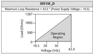
The Field Communicator requires a minimum loop resistance of 250 for communication.
