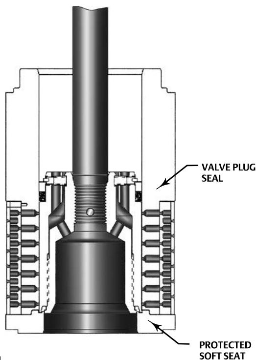
Figure 8. Cavitrol III One-Stage Cage
