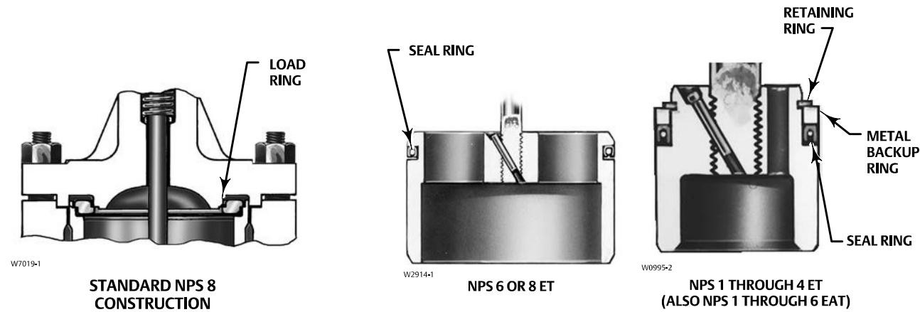
**SPRING-LOADED SEAL RING CONSTRUCTION
