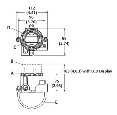
A. Standard cover B. Display cover C. LCD display
