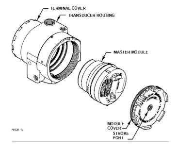
Figure 3. Master Module Construction
