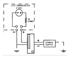
NOTE: THE 3311 IS NOT A CONSTANT RESISTOR IN SERIES WITH AN INDUCTOR. IT IS BETTER MODELED IN THE LOOP AS A 50 OHM RESISTOR IN SERIES WITH A 6-VOLT DC VOLTAGE DROP WITH NEGLIGIBLE INDUCTANCE.
