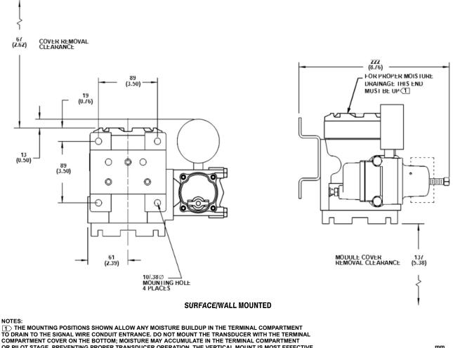
OR PILOT STAGE, PREVENTING PROPER TRANSDUCER OPERATION. THE VERTICAL MOUNT IS MOST EFFECTIVE FOR MOISTURE DRAINAGE IN WET APPLICATIONS.
