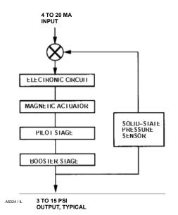
Figure 4. Functional Block Diagram
