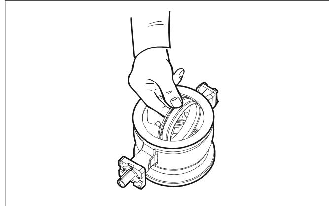
Fig. 23 Lifting the seat
