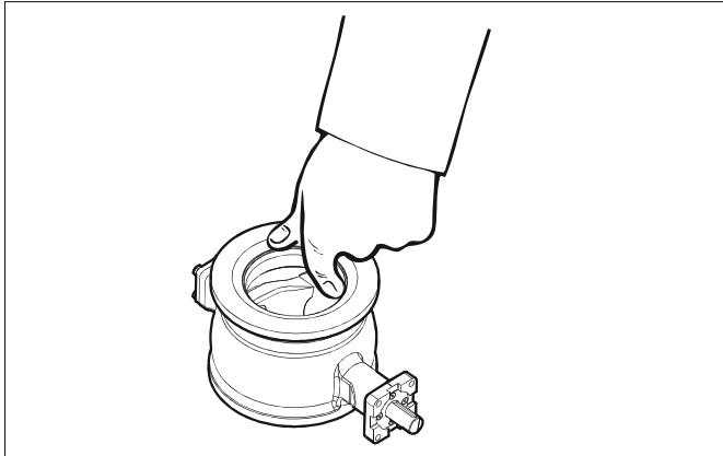
Fig. 20 Turning the ball segment
