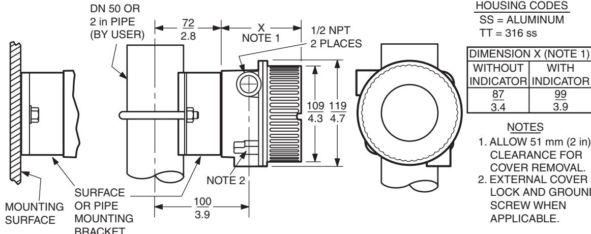
UNIVERSAL HOUSING WITH INTEGRAL SENSOR AND/OR SENSOR AND THERMOWELL
