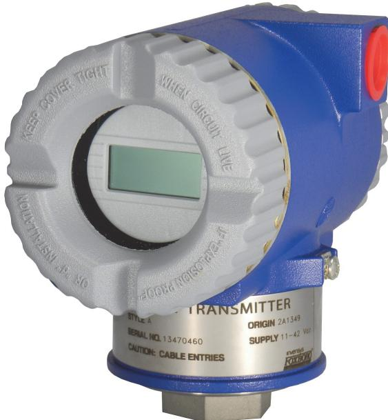
The Foxboro® brand Model RTT80 is a microprocessor-based temperature transmitter with FOUNDATION Fieldbus Communication Protocol. It receives input signals from thermocouples, RTDs, resistance (ohm), or voltage (mV) sources.
