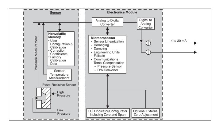
Figure 20. Transmitter Functional Block Diagram
