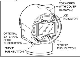
Figure 17. LCD Indicator with Pushbuttons
