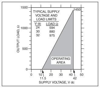
Figure 18. Supply Voltage vs. Output Load
