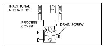
Figure 4. Vertical Mounting - Cavity Draining
