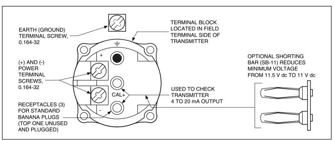
Figure 21. Field Terminal Block
