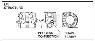
Figure 12. Horizontal Mounting with Drain Screw
