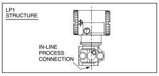
Figure 7. Low Profile Structure - LP1 Shown
