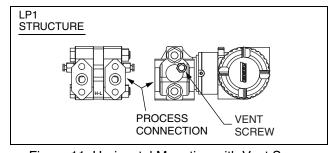
Figure 11. Horizontal Mounting with Vent Screw
