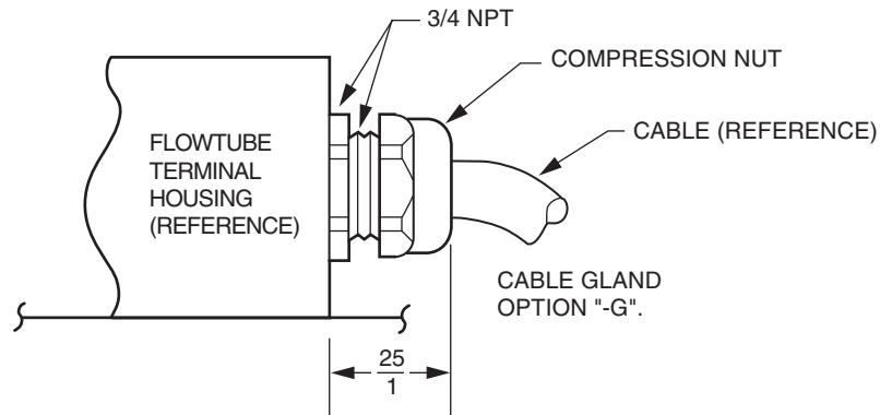
OPTIONAL SIGNAL CABLE SEAL FOR CONDUIT APPLICATIONS**mm
