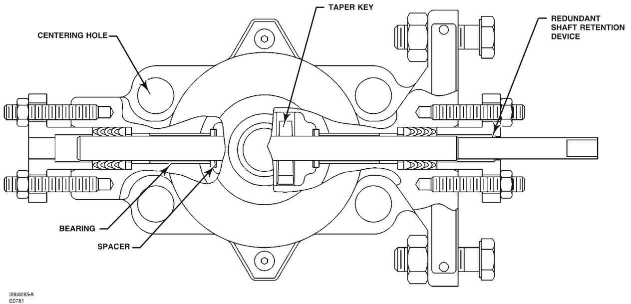
Figure 4. Typical Fisher 8510B Construction Detail with Double D Shaft
