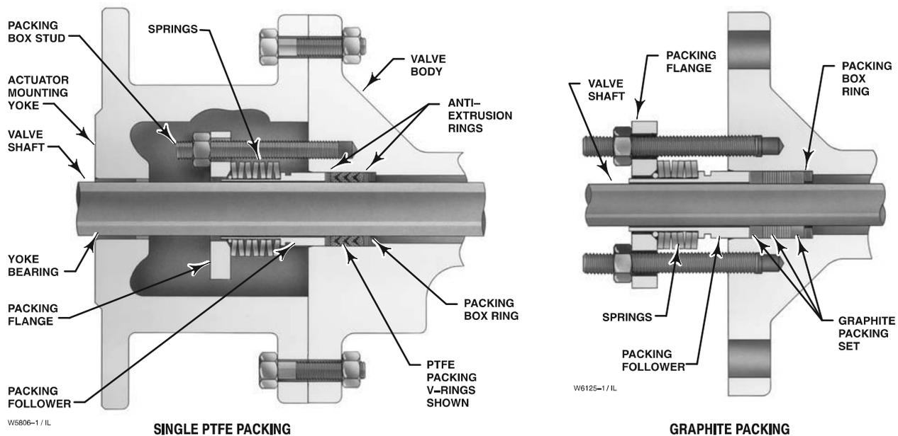
Figure 8. Typical ENVIRO-SEAL Packing Arrangements for Rotary Valves
